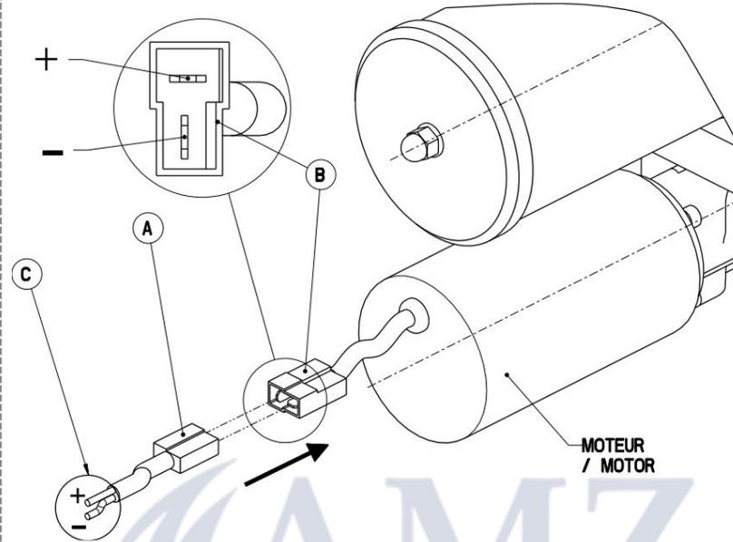
**! All the electrical connections below must be carried out once the electrical supply has been cut off.**
